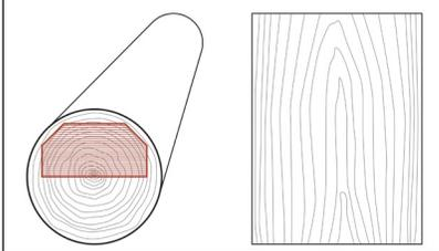
Plain slicing is the most common method of cutting a log, where the slice is parallel to the center cut of a log.
